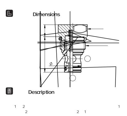
A screw-in, direct acting, poppet type check valve. Main use is as a blocking or load-holding device. The valve allows flow passage from port 1 to 2: the cartridge has a fully guided check which is spring-biased closed until sufcient pressure is applied at port 1 to open to 2. The fow is blocked in the opposite direction (2 to 1).
